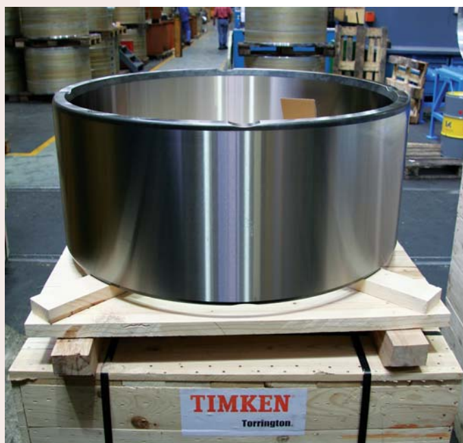
Inner race of a cylindrical roller bearing.
